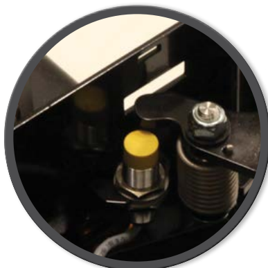
Compartment door interlock sensor
