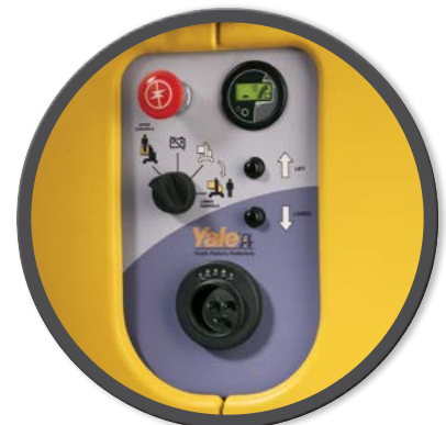
Lower control panel
