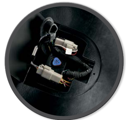
Second diagnostic panel located in the operator compartment
