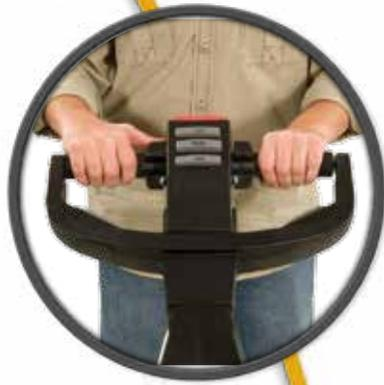
*Butterfly/twist grip combination control handle has left-hand and right-hand controls, allowing fingertip control of lift/lower, travel and horn functions with both hands.*
