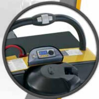
*Padded and contoured steady rest offers a soft, comfortable grab point and integrated controls.*
