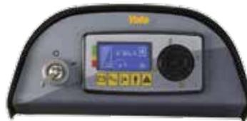
Yale iSi Technology™ incorporates a common control system with consistent functionality across the warehouse product line. The Integrated Smart Interface utilizes the same software, diagnostic codes and functionality for the main warehouse trucks creating commonality for users, supervisors and service personnel. The system offers full customization to allow a user to properly match the trucks' performance with the skill of the operator.
