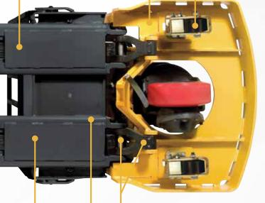
Lubrication and "x" groove bushings at all pivot points.
